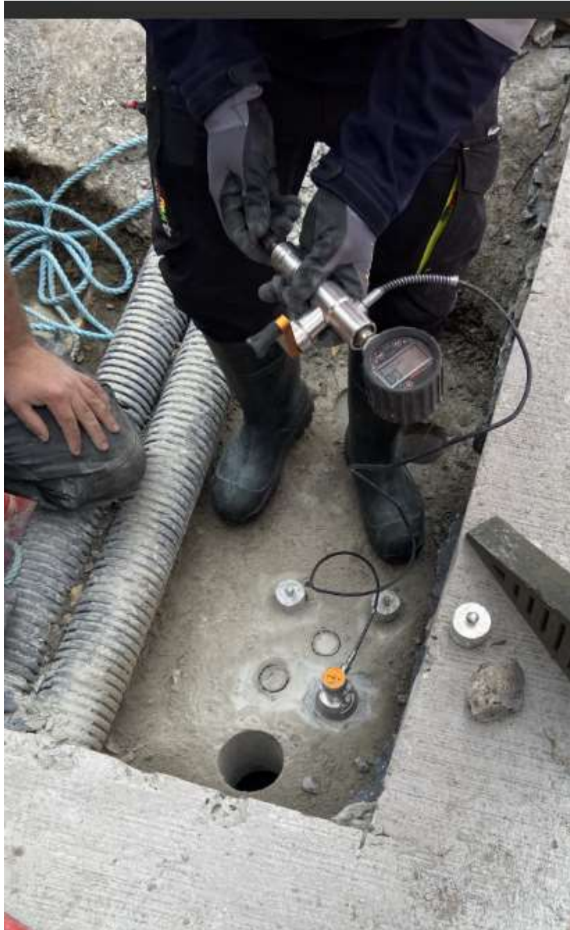
Figure 12: Adhesion test readings
